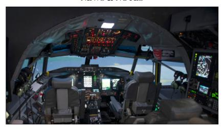
**OFFUTT RECEIVES NEW RC-135 SIMULATOR** – Pilots and navigators will now be able to train on the latest Baseline-Charlie avionics technology at Offutt Air Force Base following the recent delivery of a new RC-135 flight simulator.
